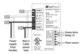
Sensor, relay and home automation connections are made to the terminal block by inserting the wires into the square openings and tightening the screws on the side.
